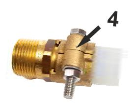
Tighten the bolt until clamp is completely closed (4). In some caseslike in cold weather when pipe is very hard tightening is good to make in several steps and keep some breaks between in attend to let pipe to get modified under the clamp.
