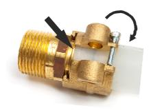
Make sure the fitting insert is pushed inside until it stops to the collar. Start opening the small expanding screw and make sure that fitting doesn't slide out on it's position. Remove the small screw completely from the clamp. This screw is for onetime use only and if clamp needs to be re-opened is better use new screw.
